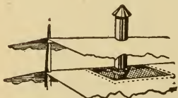
Showing Section of Double Roof and Ventilator.
