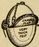
Sectional View of Water Cooling Canteen.
